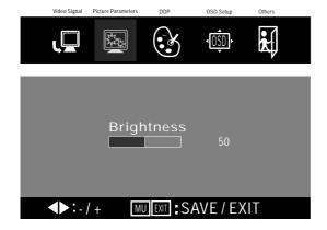
Press button 2: adjust brightness to lighter level. Press button 3: adjust brightness to darken level. Press button 1 to confirm setting. (Brightness adjustable level: 0-100. Preset: 50)
